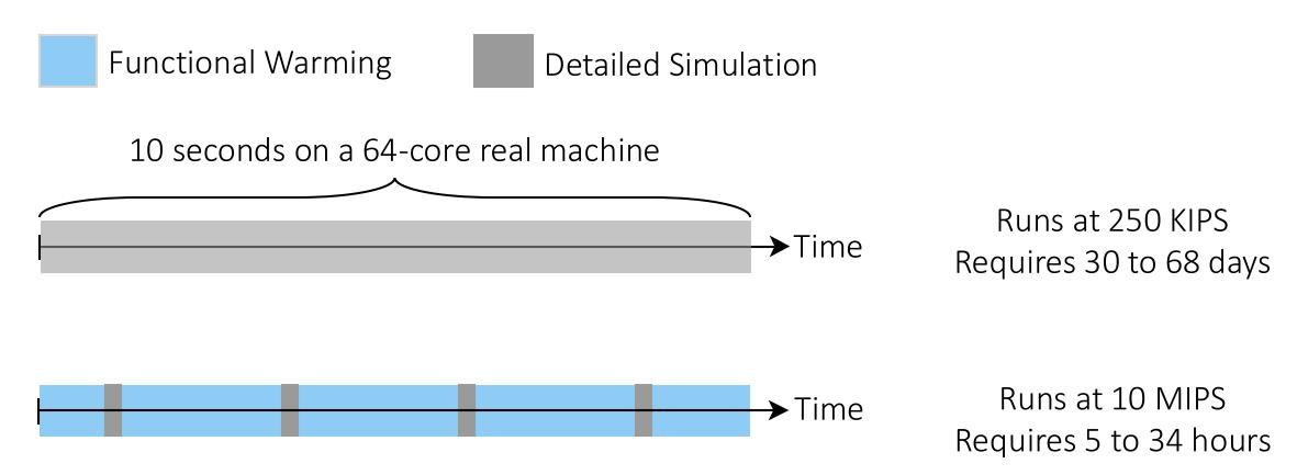
0.15% to 0.4% cycles simulated in detail and in parallel
