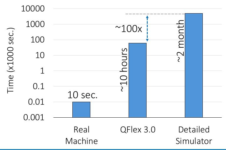
QFlex 3.0: Hour-long simulations, ~100× faster than full detailed simulation
