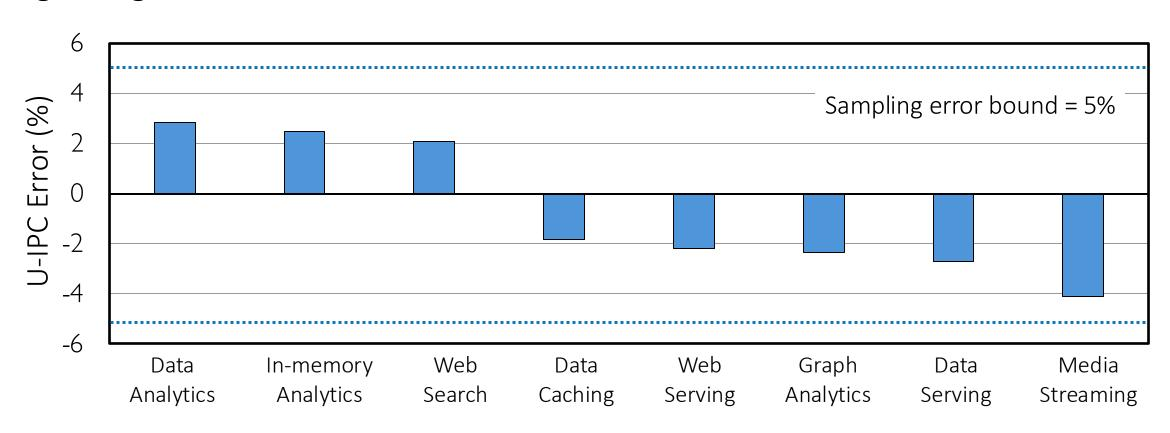
Simulation sampling's results are within 5% of detailed simulation results
